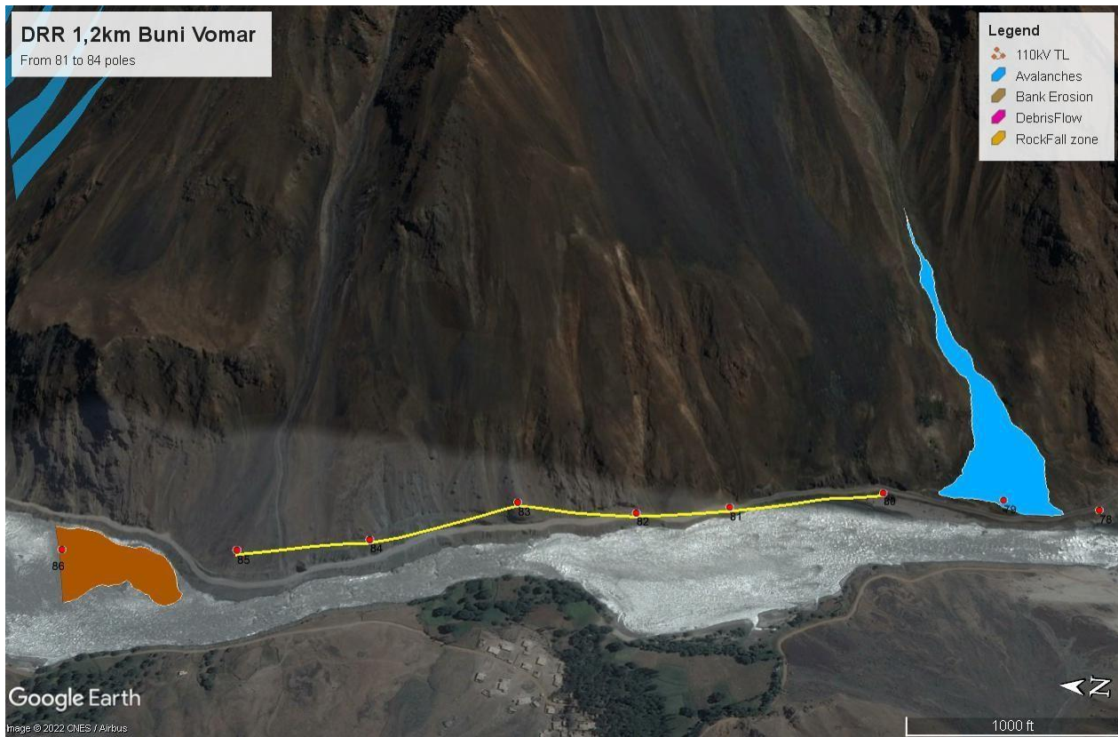
Figure 14 Natural hazards & risks along the Transmission line in the section 1.2km Buni-Vomar (poles 81-84)
